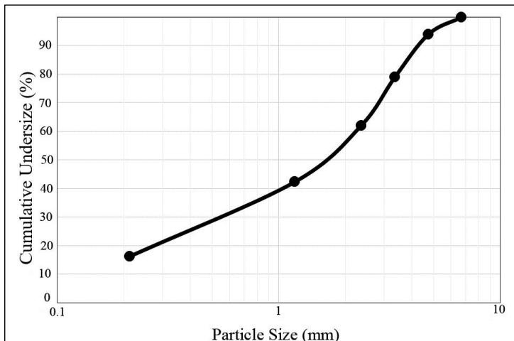
Figure 3- Particle size distribution of iron ore sample.
