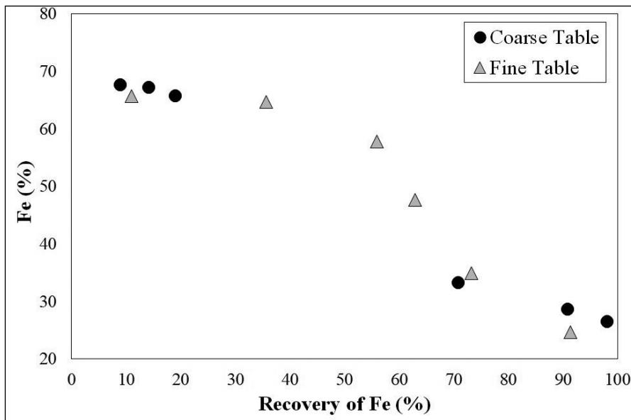
Figure 6- Grade/recovery curves of shaking table tests.
