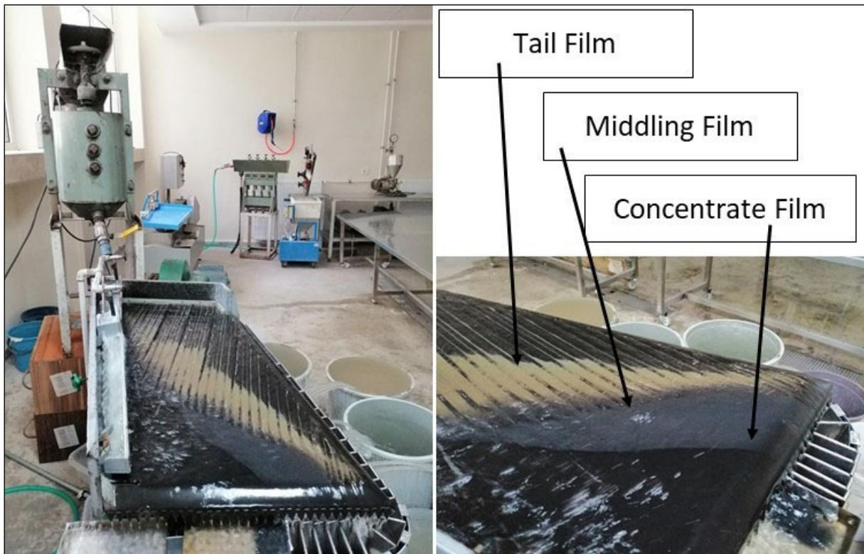
Figure 5- Shaking table test and sampling apparatus.
