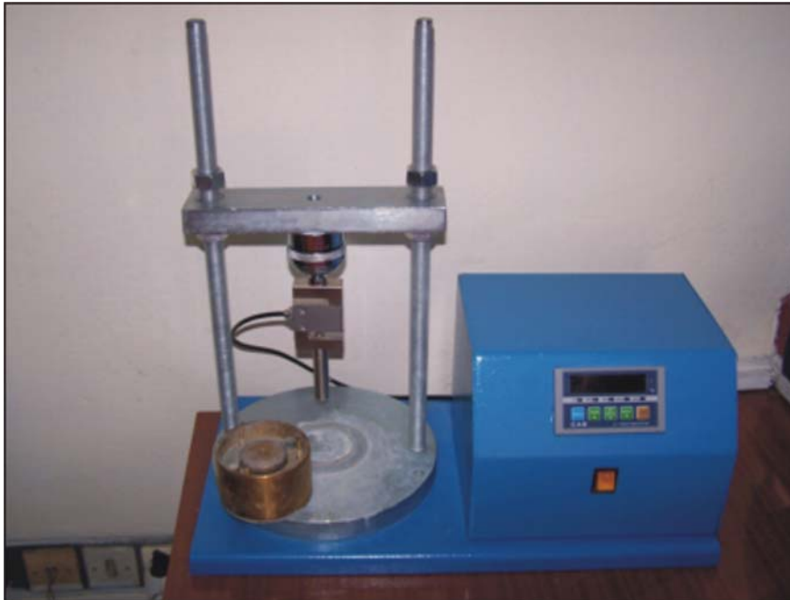
Figure 1- Constant volume swell test apparatus.
