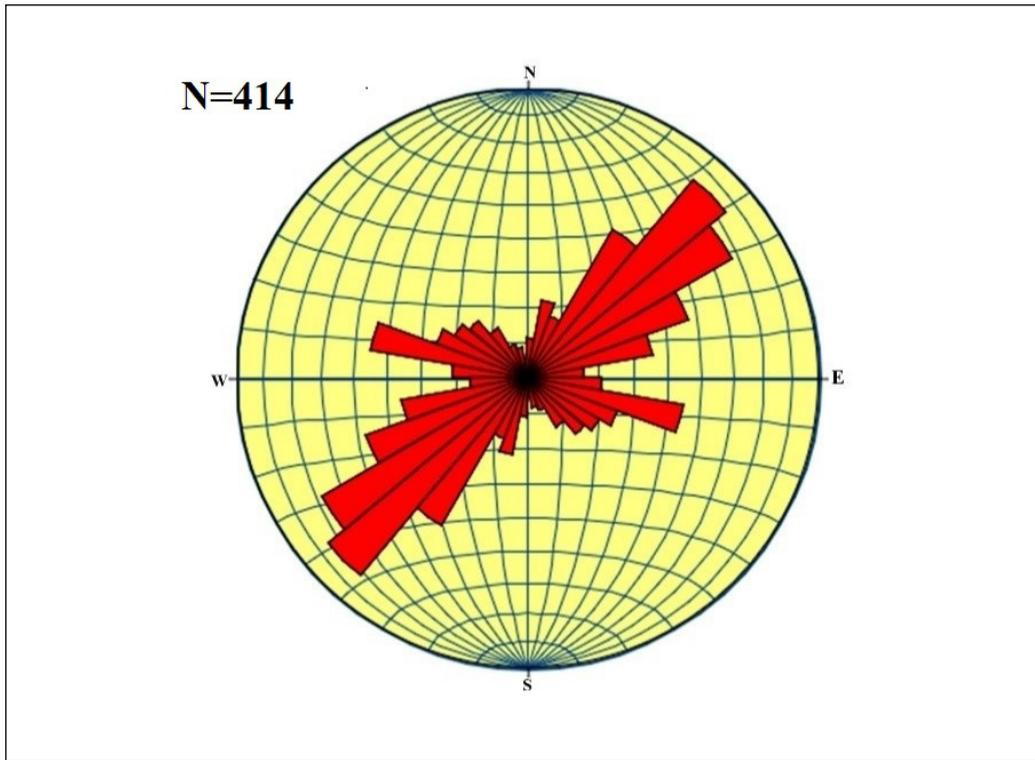
Figure 7- Rose diagram of the lineament orientation.
