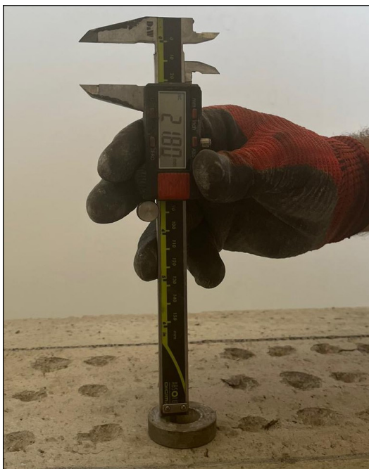
Figure 8- Measurement of nail penetration depth when a nail did not exhibit a piercing into rock.
