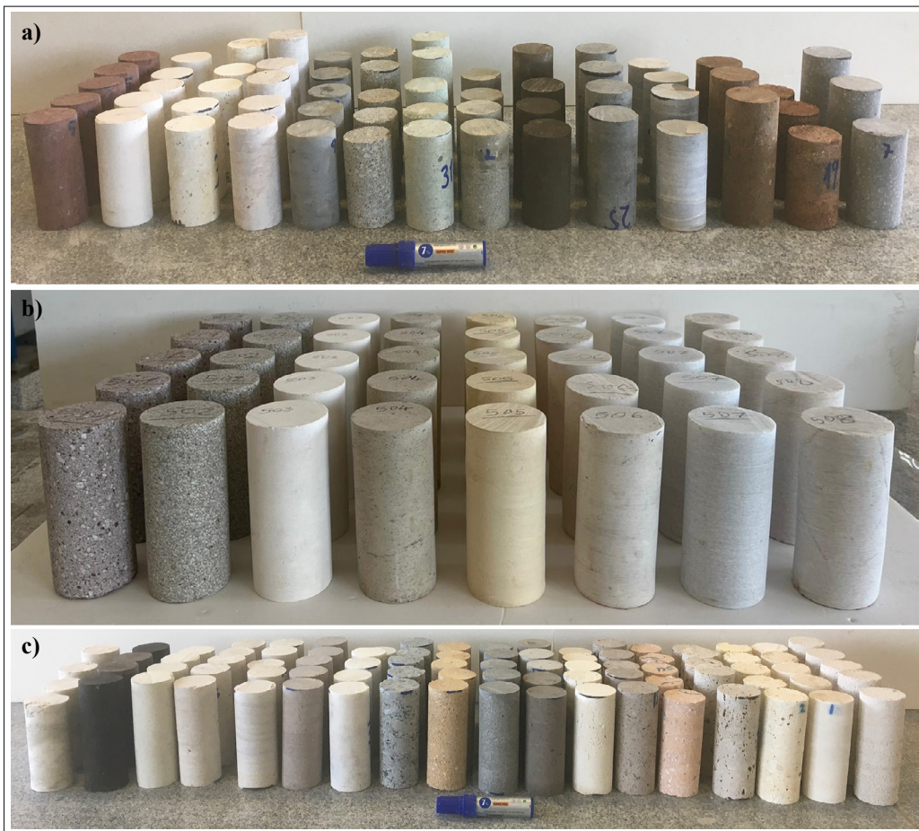
Figure 7- Core samples extracted from different rock types.
