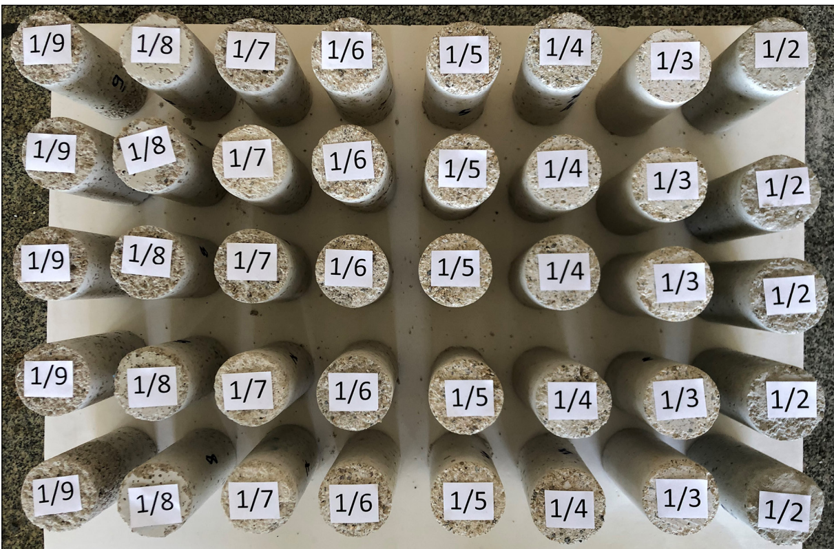
Figure 5- Core samples of concrete prepared from different cement/sand ratios.
