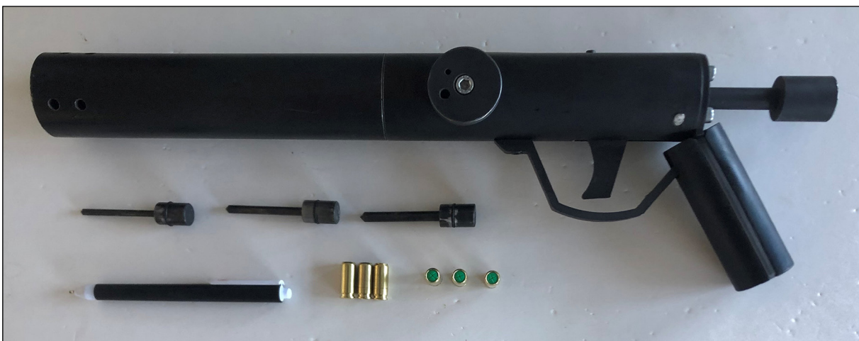
Figure 1- Nail gun, nails of three different diameters, and sound bullets used in the investigation.
