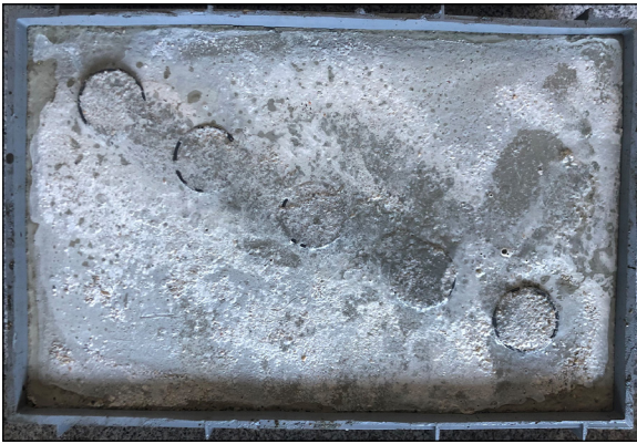
Figure 4- Casted concrete and impregnated cylindrical core samplers.
