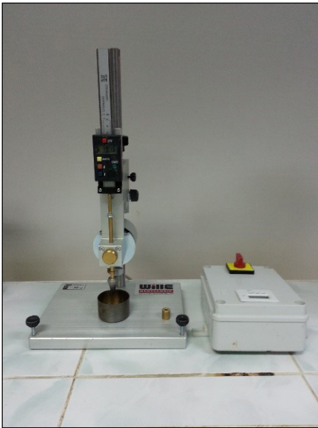
Figure 2- The fall cone device used in this investigation.
