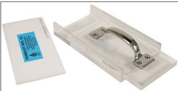
Figure 3- Roll-plate device for plastic limit tests.
