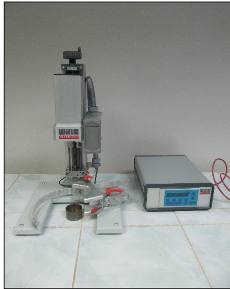
Figure 4- Miniature vane shear test device.
