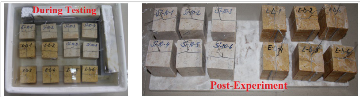
Figure 7- Visuals of samples dipped in epoxy and silane during and after the experiments.
