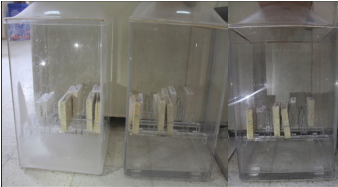
Figure 9- Image of the test for the determination of resistance to ageing by \text{SO}_2 in a humid environment.
